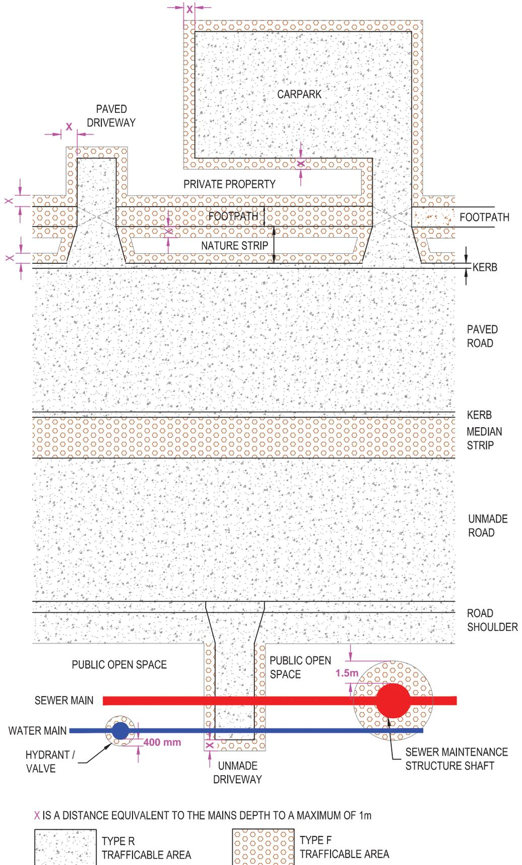
**Figure 2- Trafficable Backfill Types and Locations**
