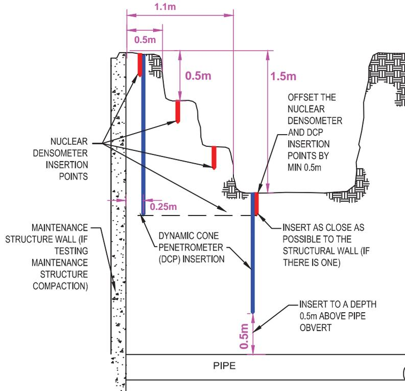
**Figure 7: Compaction testing for Deeper Pipe installations**
