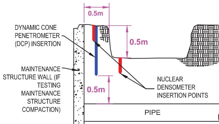
**Figure 6: Compaction testing for Shallower Pipe installations**
