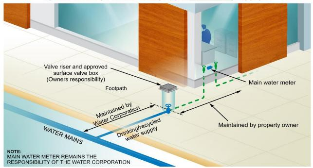
Water Corporation to maintain to the first accessible stop valve from the water main, main water meter or any part of the property service pipe is located within or beneath the walls of a structure
