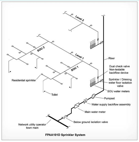
This Technical Sprinkler Specification has been developed to provide a fit for purpose sprinkler system for use in Class 2 & 3 buildings, which are a minimum of 4 storeys, and less than 25mtrs high. This system is fed from the drinking water (general) supply rather than a dedicated fire service, and includes supply for toilets in each apartment. The following points should be considered by the Fire Service Designer:
