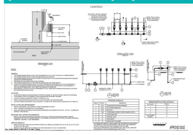
Figure 37: Multi Meter Manifold Installations Drinking & Recycled Water Arrangements
