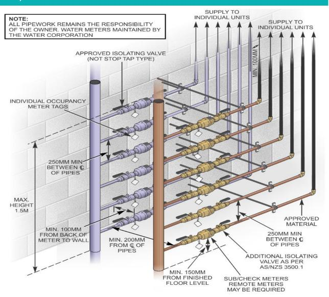
Figure 8: High Rise Sub/Check Meter Typical Arrangement Option 2 (Drinking / Recycled Water)
