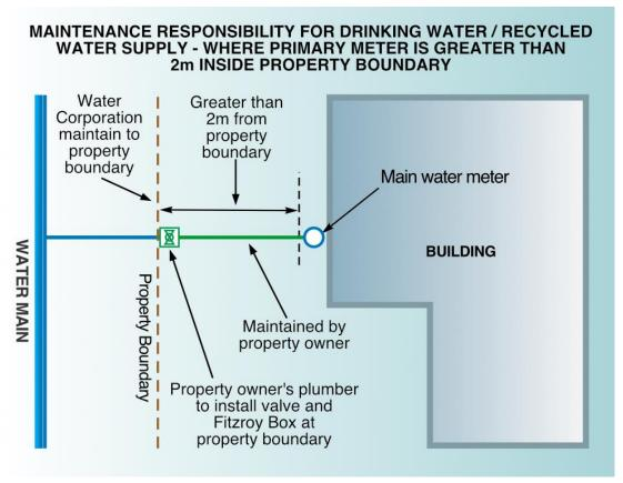
Water authority approval is required before a main water meter can be greater than 2 meters from property boundary.
