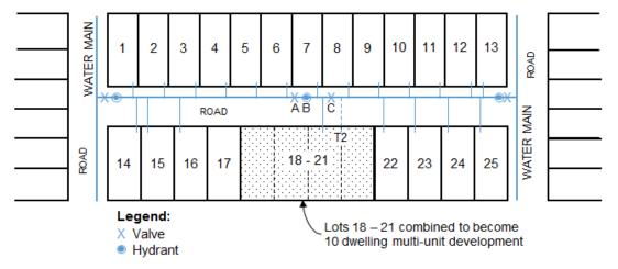
The creation of the 10 dwelling multi-unit development has resulted in a shut-off area with greater than 25 service connections. Valve 'A' is required to create shut-off areas with less than 25 service connections. Hydrant 'B' may be required dependant on the Water Corporation or Council requirements.
