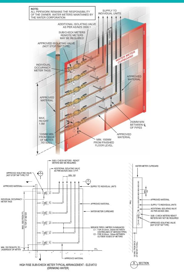
Figure 7: High Rise Sub/Check Meter Typical Arrangement Option 1 (Drinking / Recycled Water)
