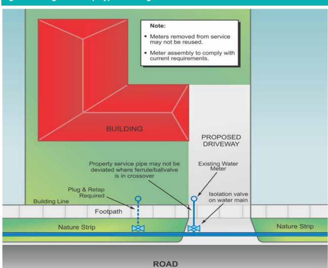
Figure 15: Plug and Re-tap Typical Arrangement
