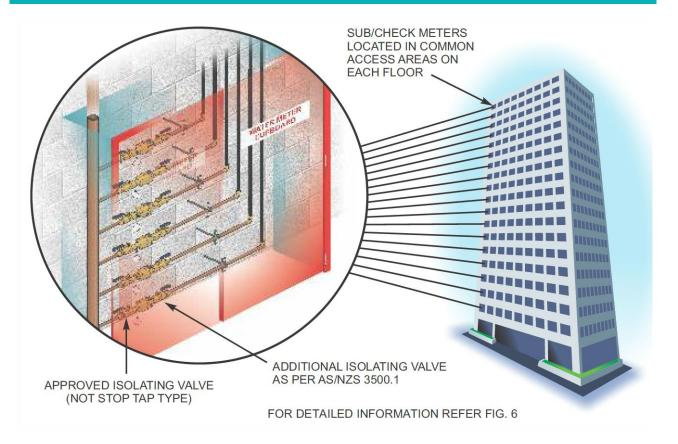
Figure 6: High Rise Sub/Check Meter Typical Arrangement
