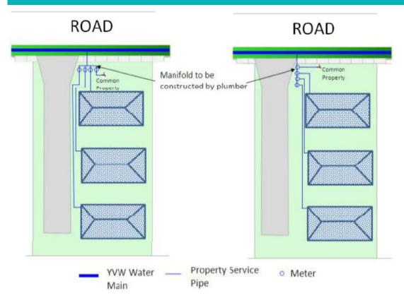
Figure 34: Typical Multi-Dwelling Residential Development with Potable and Recycled Water Manifold
